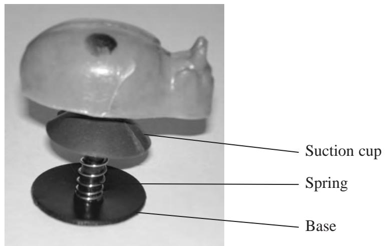
The top of the toy is pushed down, compressing the spring. The suction cup adheres to the base and holds the toy down. After a short time, the suction cup leaves the base, causing the toy to jump.
